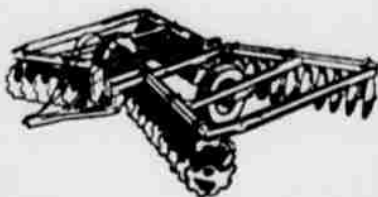
MF 52 Pull-Type Wheel Disc. Sealed ball bearings never need greasing. Heavy-duty adjustable hitch with automatic leveling linkage. Adjustable gang angle and spread. Heavy wrap-around frame, 3 sizes: 10 ft. 9 in., 12 ft. 3 in., 13 ft. 8 in.
