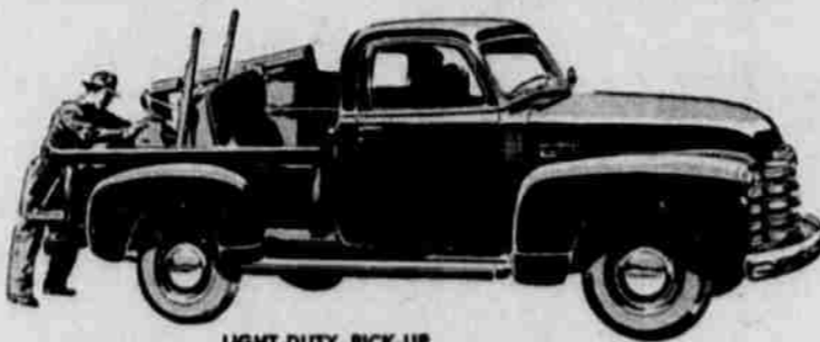
LIGHT-DUTY PICK-UP Model 3704—116-inch wheelbase, Maximum G.V.W. 4,600 lb. Other models available: 3604—125 1/4-inch wheelbase, Maximum G.V.W. 5,800 lb; 3804—137-inch wheelbase, Maximum G.V.W. 6,700 lb.
