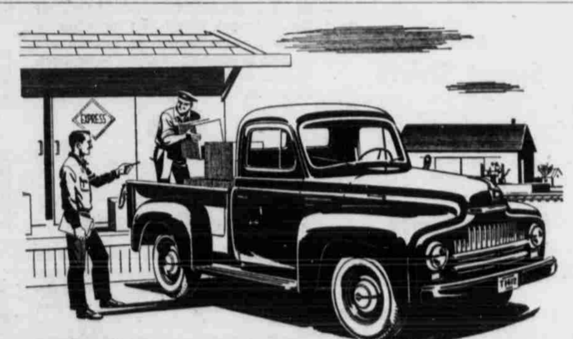
Model L-110, 115-inch wheelbase, 614-foot pickup body, 4,200 lbs. GVW. Pickups in the L-110, L-120 and L-130 Series include 115, 127 and 134-inch wheelbases, 6 1/2, 8 and 9-ft. bodies, GVW's to 8,600 lbs.
