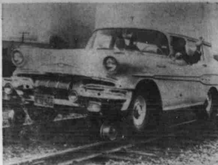
TRIPPING THE RAILS IN A CAR - Los Angeles, Calif. - Here's an auto that's at home on a railroad track or a highway. It's called the Fairmont Hy-Rail Motor Car and it has been in use, by the Southern Pacific, on railroad tracks and on regular streets, for about a month. The car is said to be useful in line inspection but with highways becoming more crowded by the day—who knows where it might lead.
