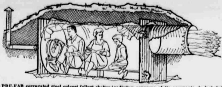
**PRE-FAB corrugated steel culvert fallout shelter for three persons can be bought for about \$150, plus delivery and installation. The shelter, which would cut to 1/500th the amount of outside fallout radiation exposure of its occupants, is included in the "Family Shelter Designs" booklet now at state and local civil defense offices for public distribution. It is available without charge.**
