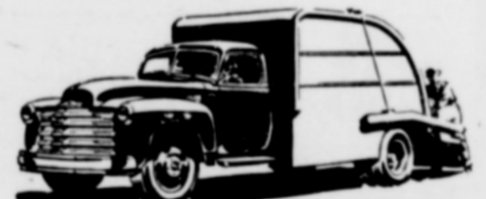
HEAVY-DUTY CAB-AND-CHASSIS with Refuse Body Model 6403—161-inch Wheelbase Maximum G.V.W. 16,000 lb.
