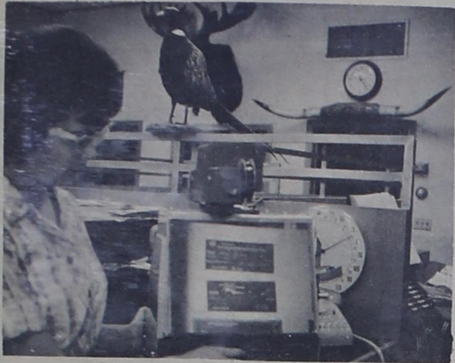
Mrs. Beverly Dillard effectively displays the Recordak Film Reader which is a machine designed to read the film of the checks that are filmed on the Microfilm.
