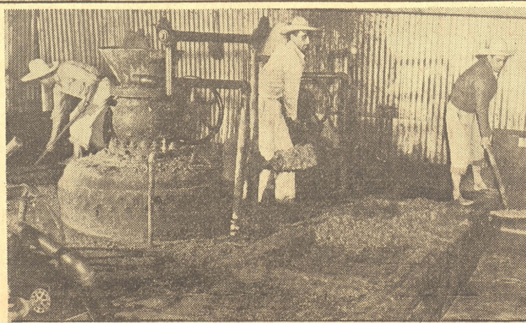
Here the shredded shrub is being placed in old-fashioned rotating drums where one step in the separation of the rubber is accomplished. To increase the production of rubber for use in the American War program, the General Tire & Rubber Company has announced plans for a guayule project in Mexico and will erect an extraction mill in the heart of the guayule area in the state of Coahuila.
