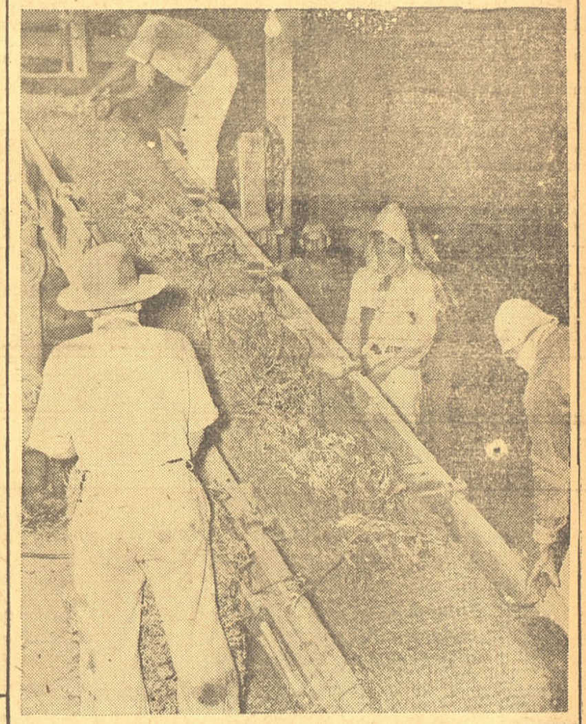
This belf carries the guayule shrub, root and all, into steel rollers, where they are shredded before being placed in rotating drums or pebble mills. The General Tire & Rubber Company plans on introducing modern American methods and machinery to replace the system which has been in use since the guayule industry got its start 50 years ago.
