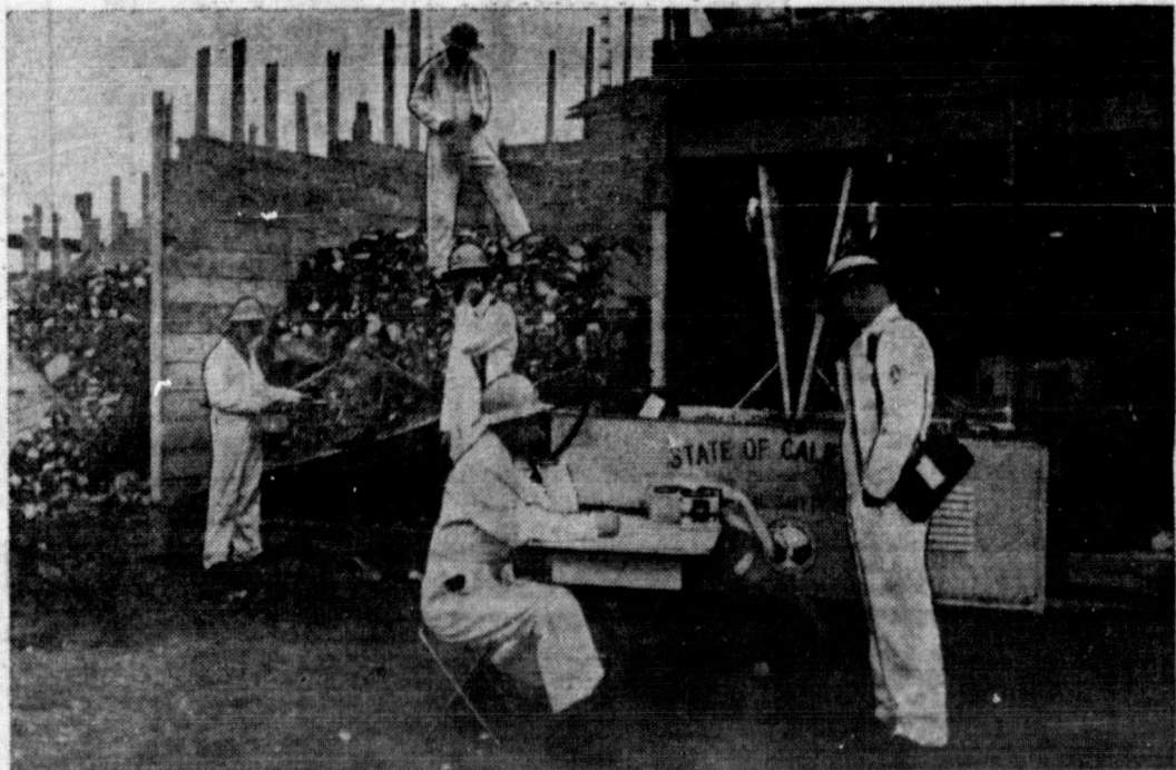
RADIOLOGICAL MONITORS of the San Diego City-County Civil Defense organization go through their paces by checking on "fallout radiation" at a training site designed specifically for civil defense use. After taking their readings, the men in background would radio their reports to a central plotting and coordinating crew such as the two manning the radiological trailer in foreground. The nation's radiological monitoring capability is being expanded rapidly by civil defense at all levels, including more than 15,000 monitoring stations now operating. (OCDM Photo)
