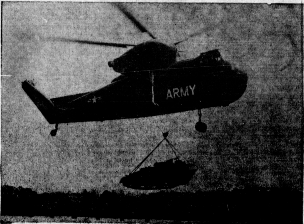
ARMY'S BIGGEST —The twin-engine, all-metal H-37 "Hoyax" helicopter was designed to carry 36 combat soldiers, evacuate 24 litter patients, or carry cargo. As the Army's largest helicopter, it's a "going concern" in Transportation Corps helicopter companies available to support units of the pentomic Army. Here it easily carries a 15,000-lb. "Scorpion," a full-tracked, self-propelled armored vehicle which mounts a high-velocity 90mm anti-tank gun.
