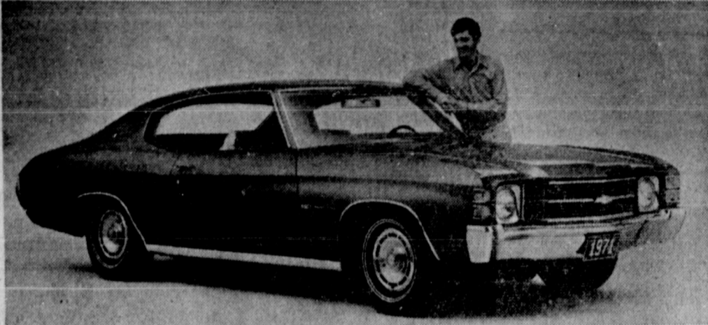
Single-unit Power-Beam headlamps and a new grille and front fender lamps incorporating parking, turn signals and side marker are features of the 1971 Chevelle. Chevelle continues to be the industry's top selling intermediate car. This Malibu model has hidden windshield wipers, full door-glass styling and Astro Ventilation with vent-ports on the instrument panel. In 1971, SS equipment is available on the Malibu Coupe and Convertible with any optional V8 engine. Chevelle and other new Chevrolet models go on sale on Tuesday, September 29.
