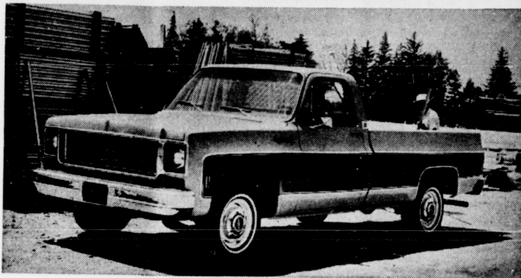
Completely restyled and with extensive chassis redesign, the 1973 Chevrolet pickup features many improvements in appearance, comfort, durability, and ride and handling for both commercial and personal transportation. Highlights are curved side windows, highly-styled interiors, powered flow-through cab ventilation, new leaf-spring rear suspension, increased engine cooling capacity, outside fuel tank, and easier servicing. Wheelbases are increased for better load distribution.
