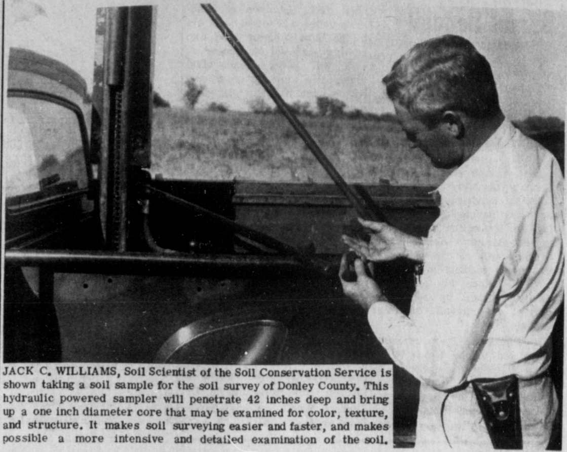
JACK C. WILLIAMS, Soil Scientist of the Soil Conservation Service is shown taking a soil sample for the soil survey of Donley County. This hydraulic powered sampler will penetrate 42 inches deep and bring up a one inch diameter core that may be examined for color, texture, and structure. It makes soil surveying easier and faster, and makes possible a more intensive and detailed examination of the soil.
