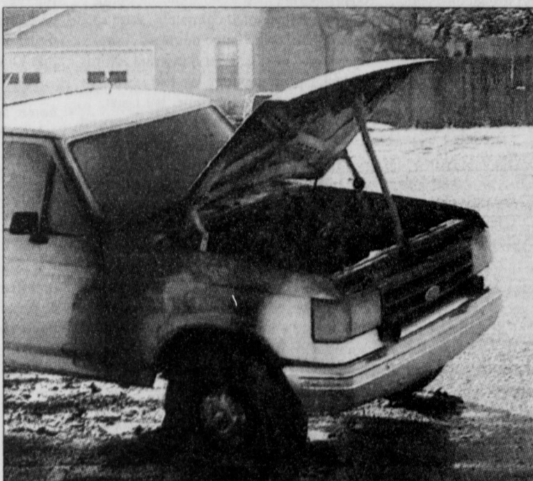
A fire burned up the engine compartment of CHS junior Shane Gayle's truck early Tuesday morning. Gayle said he thought the power steering line came loose and was ignited by the manifold. Enterprise Digital Photo.
