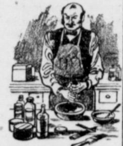
The ink used by CURRIER & IVES for their prints was composed of BEEF SUET, GOOSE GREASE, WAX, SOAP SHELLAC, GUM MASTIC AND GAS BLACK..
