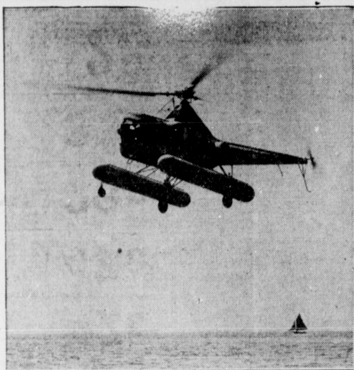
RESCUE SHIP OVER LAND OR SEA —With its new wheels prominently displayed, the Air Force's first amphibious helicopter, the H-5H, is shown making a routine over-water flight. The wheel-float combination greatly increases the H-5H's utility as a rescue, search and liaison aircraft, allowing it to land with equal facility on land or water. The ship is equipped with a hydraulic winch, and when terrain or rough seas make it impossible to land, it can hover motionless over the area and haul survivors up into the cabin.
