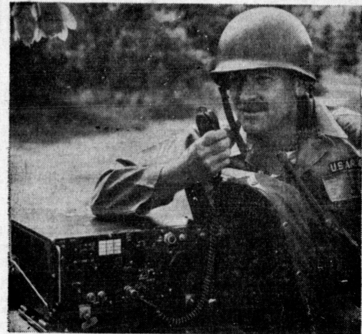
THE AN/VRC-12 , the U. S. Army's new mobile, transistorized radio communications system is demonstrated by Sfc Ewen MacDiarmid (Sacramento, Calif.) of the U. S. Army Signal Research and Development Command, Ft. Monmouth, N. J. Developed by the Army Signal Corps, the VRC (Vehicular Radio Communication) system provides for voice communication among tanks and similar vehicles up to 25 miles distance and covers 920 different channels. Weighing approximately 102 pounds, the VRC is produced for the Army by the Avco Corp., Cincinnati, O.
