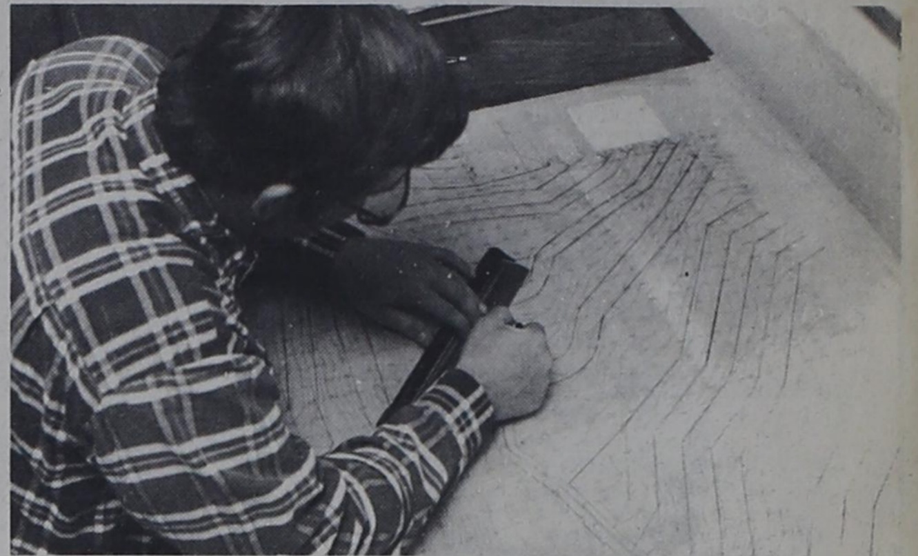
Soil conservation Technician Phil Longan completes a plastic overlay of a terracing project following actual shooting of contours and plotting of elevations. The difficulty comes with matching equal elevations while creating terraces that will accommodate farm machinery without impeding their use.
