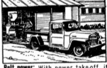
Belt power: With power take-off, it serves as a power unit for operating many types of belt-driven equipment.
