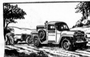
Welding: With power take-off, it supplies power to operate welders, compressors, generators.
