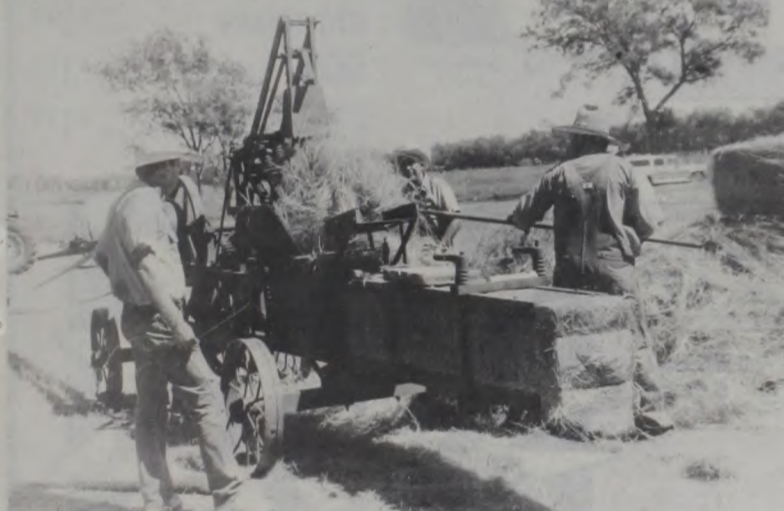
TWO HAY PRESSES or balers were only a few of the many antique farm equipment demonstrated at last weekend's show in Lindsay. The baler, above, is belt-driven by a tractor and the press, at left, is mule-powered. Janie Hartman Photos
