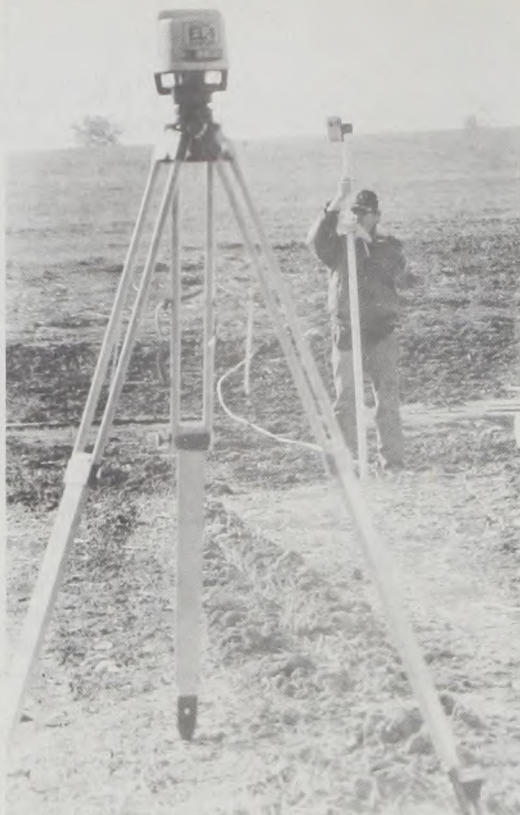
GREG TOMPKINS from Cooke County Soil Conservation surveys terraces recently constructed under the Soil District's supervision on the Kenneth Klement farm near Hood. Janie Hartman Photo
