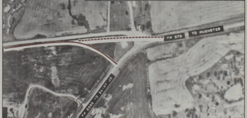
THE ONLY CONTROVERSY in the Red River Bridge project seems to be the junction with the existing highway near Bulcher. The Highway Department proposed a route indicated by the solid brown line. Muenster wants a route similar to the dotted line. The Muenster preference would allow smoother traffic flow onto FM373. Department officials at the meeting did not explain why they wanted the "T" junction. (Photo taken from aerial photo on display at the hearing.)
