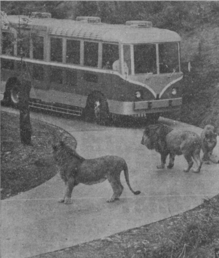
The Tama Natural Zoo in the western suburbs of Tokyo provides what approximates the natural habitat for animals instead of the usual cages. Twelve African lions roam freely, while a heavily-reinforced bus conveys visitors over the roads in the walled compounds. The roof of the bus is strong enough to withstand the pressure of four mature lions leaping simultaneously on it, and the double, full-view windows are bullet-proof as in modern army tanks.
