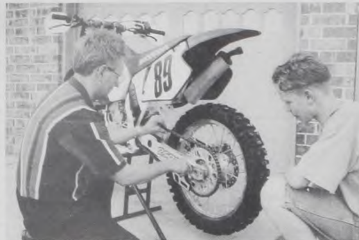
LARRY EBERHART shows Brian Wiese how to apply proper tension to a motorcycle chain, one of the many maintenance procedures Eberhart will cover in his teen class: Small Gasoline Engines-Operation, Maintenance & Troubleshooting. For more information, call the NCTC Continuing Education Office at 668-4272. NCTC Courtesy Photo
