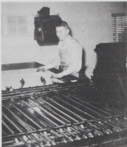
ALVIN HARTMAN hand-feeds newsprint sheets into the Meihle newspaper press at The Muenster Enterprise in the early 1950s. Photo courtesy Regina Pels
