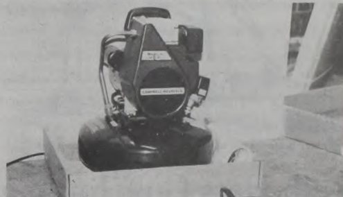
2 H.P. Air Compressor - Pancake style / Decatur Lumber Co
