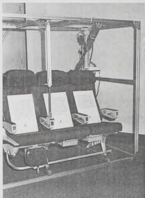
Stress test machinery was on display on the tour of Weber's new facility. Weight movement and twisting stress is repeatedly applied to seats to determine safety and durability. Tour guide Jeff King agreed with Michael Curtsinger of "Aircraft Interiors" magazine, "When people walk away from potential airliner disasters, it's because of this kind of testing." Sam Sparkman is Weber's director of safety testing and certification. Dave Fette Photo
