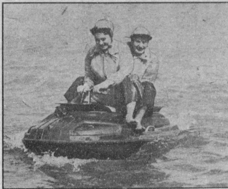
AWAY ALL SCOOTERS —Two adventurous ladies plan to cross the English Channel the "easy" way—on a water scooter. The show girls, Kay Harris, front, and Una Denton, will scoot from Calais to Dover—they hope. The machine has a speed of 20 knots, and will automatically slow and circle back if the riders fall off. The pair is shown, above, on practice run at Folkestone, England.
