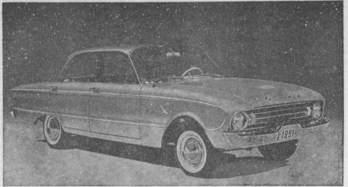
The 1961 Ford Falcon, most successful new car in history, features a new convex-shaped aluminum grille and new optional, 101-horsepower engine, but preserves the styling, maneuverability, interior roominess and 23.7-cubic-foot luggage capacity of the 1960 model. Shown above is the 1961 Falcon Fordor Sedan. Continuing its proven economy reputation, the 1961 Falcon will deliver up to 30 miles per gallon on regular grade fuel, goes 4,000 miles between oil changes, and introduces new and longer lasting bright trim and underbody parts, including a double-wrapped aluminized muffler.
