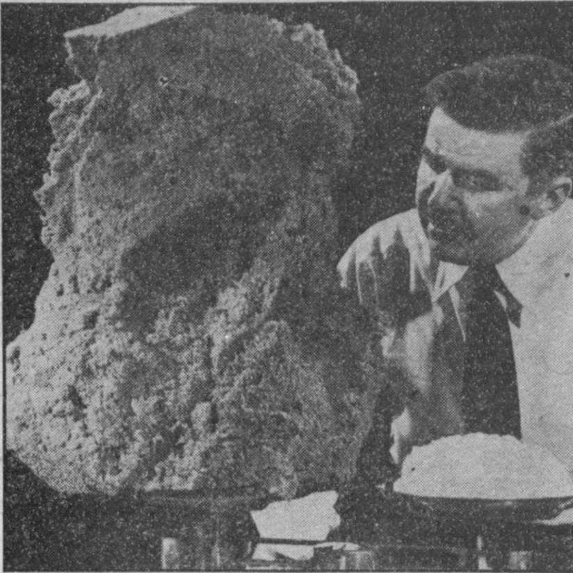
Robert Sterling, Westinghouse chemist who developed the substance, compares a chunk of his new lightweight plastic with a panful of fluffy pie meringue. Despite the difference in mass, the two balance each other at five ounces. Termed "the world's lightest solid," the new plastic foam was developed for use as an insulating material. One of its chief advantages is that it can be transported in liquid form and foamed into place wherever needed, thus saving considerable shipping space.
