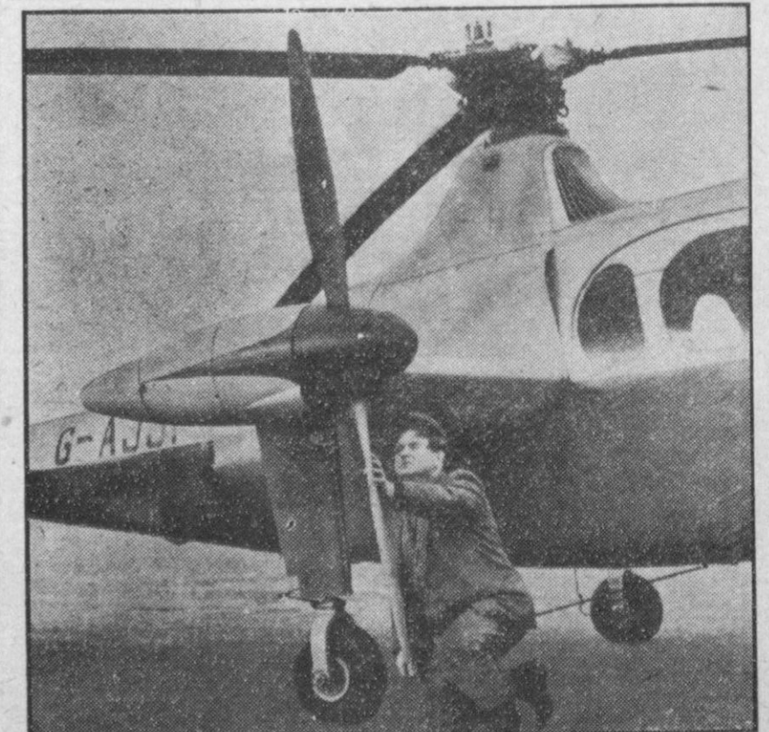
This new Fairley Gyrodyne helicopter has a stub wing with a propeller that provides most of the forward propulsion, while the main rotor keeps the aircraft aloft. The rotor aircraft has a cruising speed of 115-120 mph., and is said to be ideal for inter-city flights, air charter work and crop spraying.
