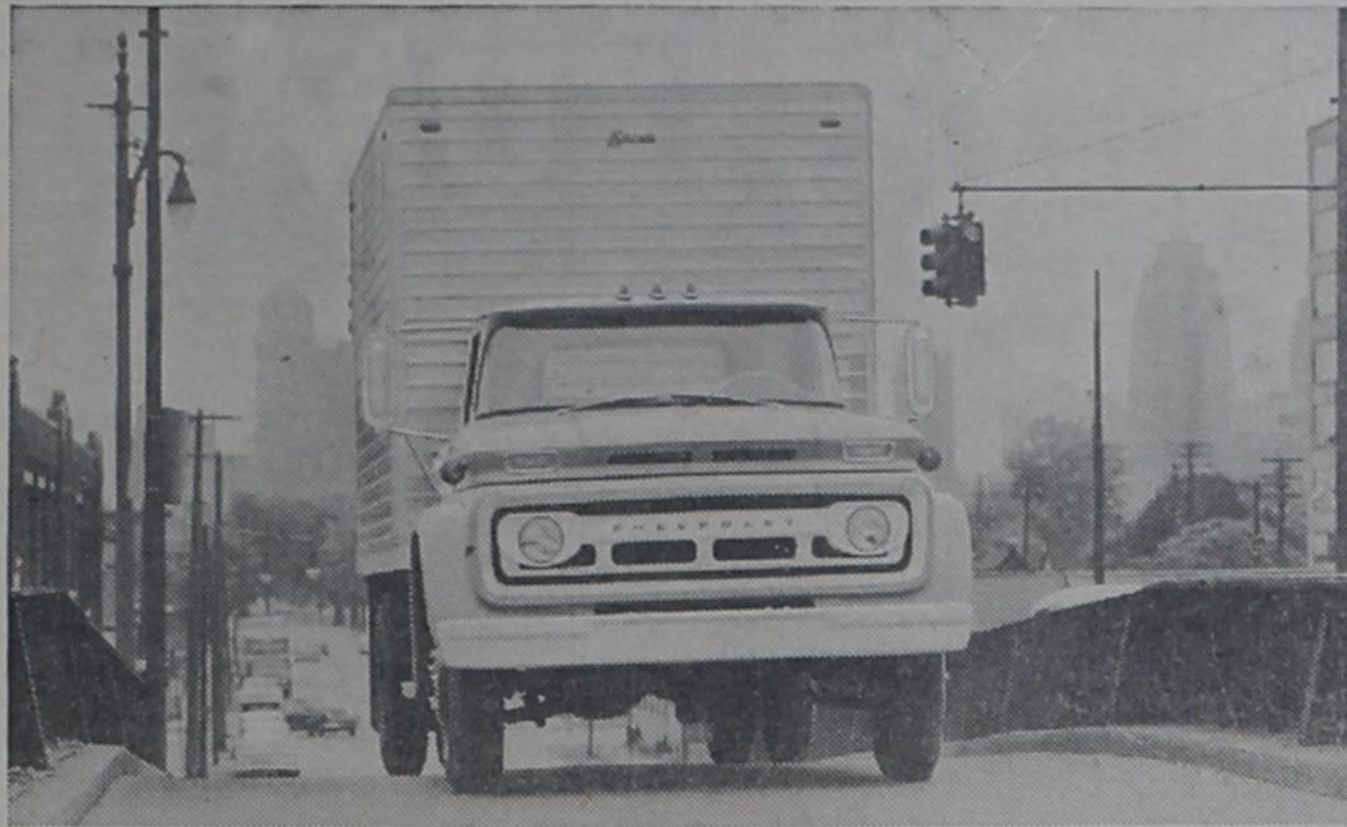
Diesel power for the first time, addition of two headlamps and longer life mufflers. New optional equipment includes alternating current generators, tinted glass and sliding rear cab window for better ventilation. Proved independent front suspension is retained with improvements.
