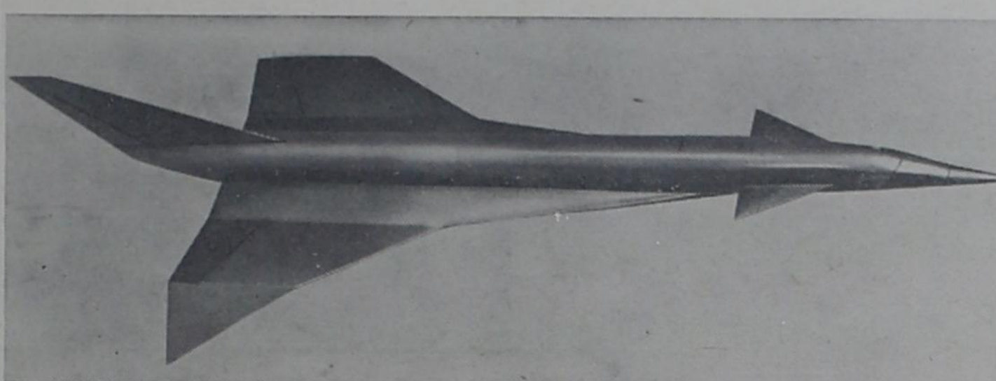
OBJECT DART —This artistic dart shaped aircraft will be a project for the future. The aircraft will carry from 100 to 130 passengers at three times the speed of sound. The plane, which company engineers say is feasible today, could be ready by 1970.
