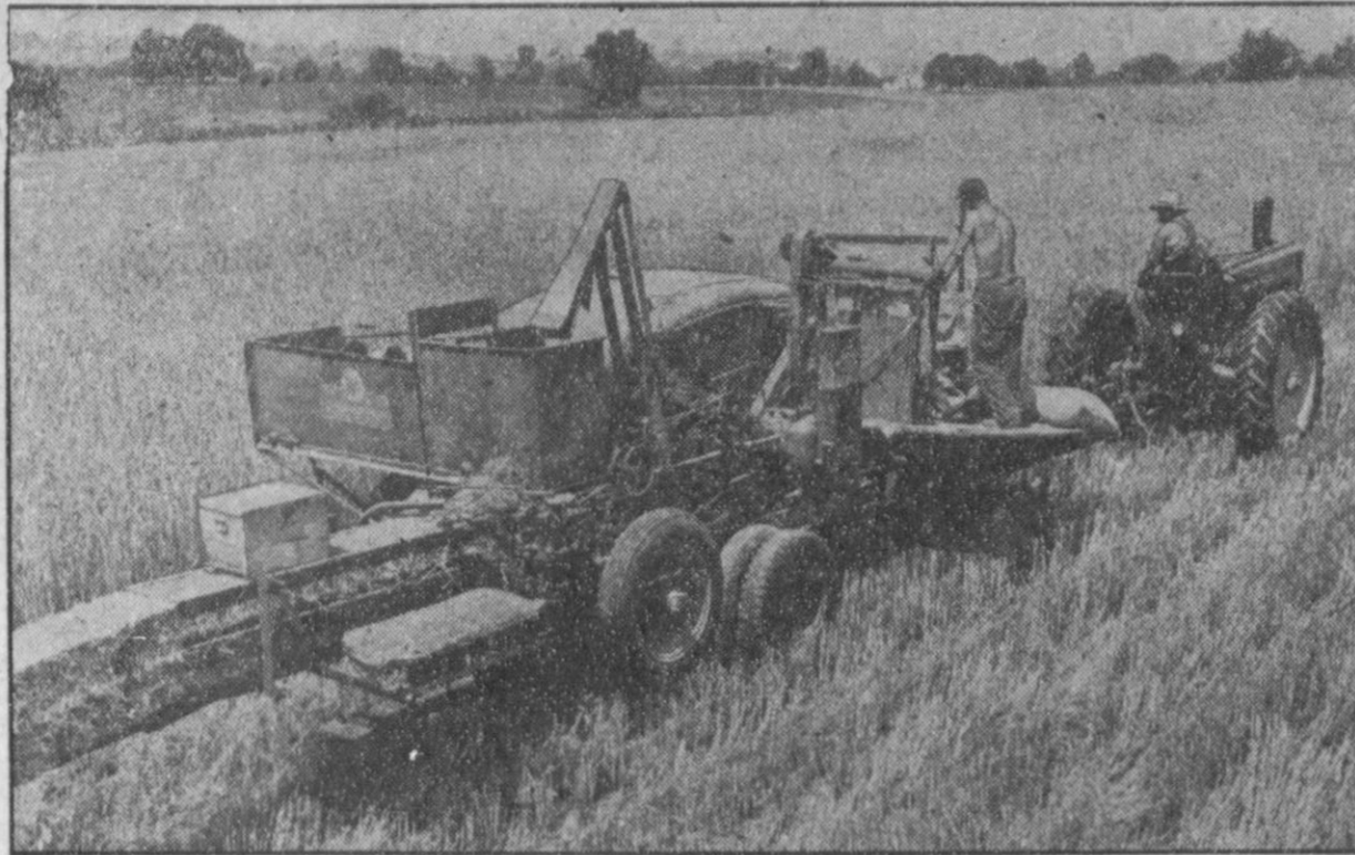
COMBINE COMBINES OPERATIONS —This machine is the latest idea in speeding up the harvesting of the nation's biggest peatime wheat crops. A standard automatic twine-tying baler was joined with a combine to do several jobs at once. With the arrangement, a two-man crew can cut the ripe wheat, thresh it, bag it, and bale the leftover wheat straw in one continuous operation. At the left an automatically twine-tied bale is shown ready to drop from the baling chamber.
