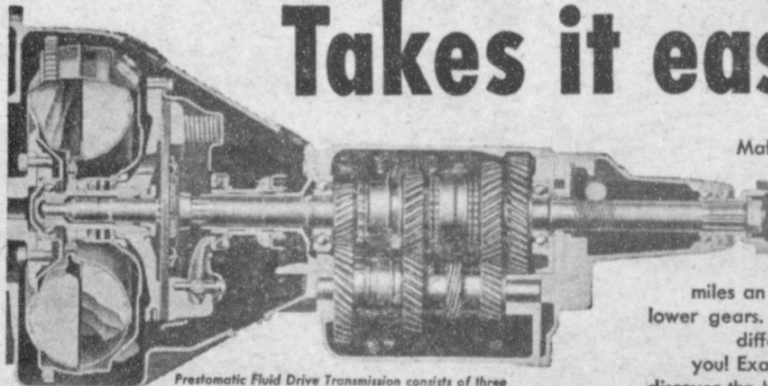
Prestomatic Fluid Drive Transmission consists of three compact units... gyral Fluid Drive, the Safety Clutch and Prestomatic Transmission. Each unit is designed with a minimum of moving parts, and each unit is ruggedly built to give trouble-free service for the lifetime of the car.
