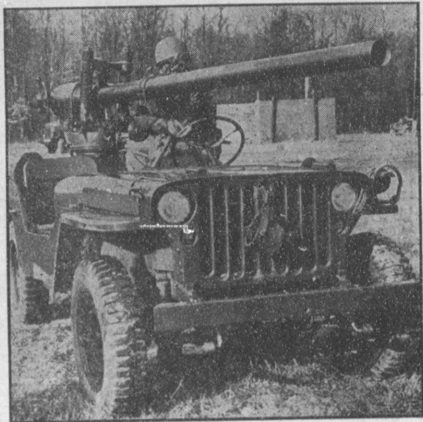
MIGHTY PEACE PIPE—U. S. Army personnel unveiled a jeep-mounted 105-mm. recoilless rifle during recent tests at the Aberdeen Proving Ground, Aberdeen, Md. Capable of knocking out any known tank, including Russia's famed 57-ton thick-armor model, the "stovepipe on wheels" ranks as the Army's mightiest tank-buster.
