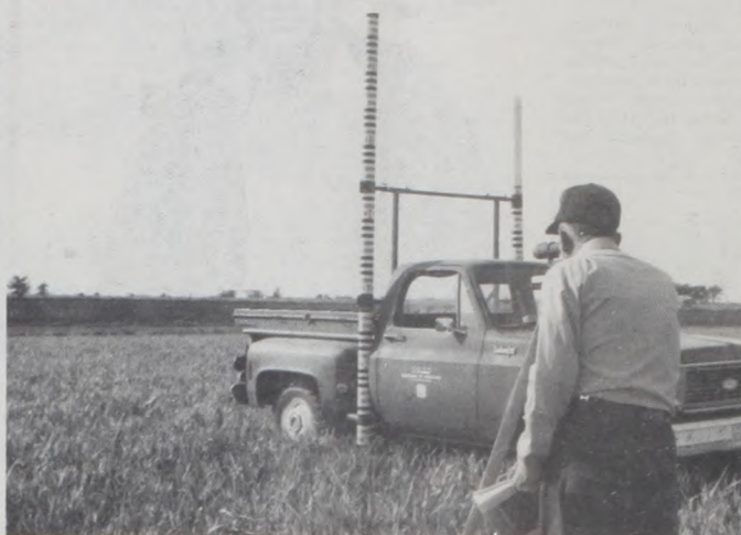
Ray Endres, civil engineering technician, is taking rod readings to be placed on a topog map. The field is divided into a checkerboard pattern with elevations being taken on 100 foot squares. The large graduated rods mounted on the sides of the pickup make this step in terrace design much faster by making these shots possible without walking the field.
