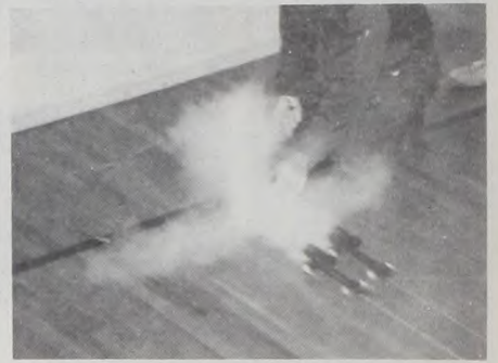
Junior high shop students line up the carbon dioxide powered mini-cars they built in class for a race in the MHS gym. The two fine lines on the floor are cords used as guides to keep the cars on a straight course. Lower picture shows the jet propelled cars blasting away from the starting line.
