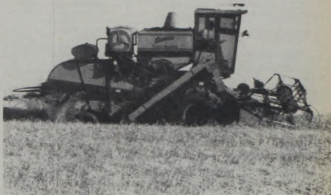
Many combines are specially equipped this season to pick up grain that was bent low by rain and wind. The device, replacing the standard reel, is set lower and has pick-up prongs rather than paddles to deliver straw to the platform. Its original use was for combining soy beans. Janie Hartman Photo
