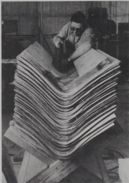
ELMO SELF fastens cutting pattern to rough form-pressed plywood which will form the seat and back of a Uniflex stackable seat.
