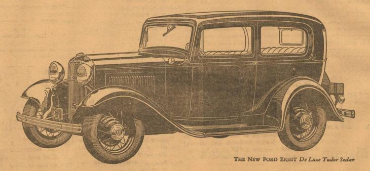
Eight-cylinder, 90-degree V-type, 65-horse-power Engine \* Vibrationless Roomy, Beautiful Bodies \* Low Center of Gravity \* Silent Second Gear Synchronized Silent Gear Shift \* Seventy-five Miles per Hour \* Comfortable
