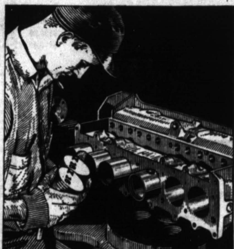
Chevrolet pistons are weighed individually, matched in sets of six to within one-half ounce, and fitted by hand to three one-thousandths of an inch clearance. Piston pins are individually tested for size on special micrometer gauges.
