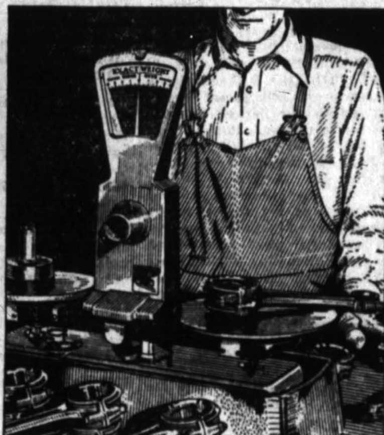
Chevrolet connecting rods are matched in sets of six to within one-quarter ounce, and are individually fitted by hand to the crankshaft. Bearings are of Babbitt metal cast into the rods under heavy air pressure and at 800 degrees Fahrenheit.
