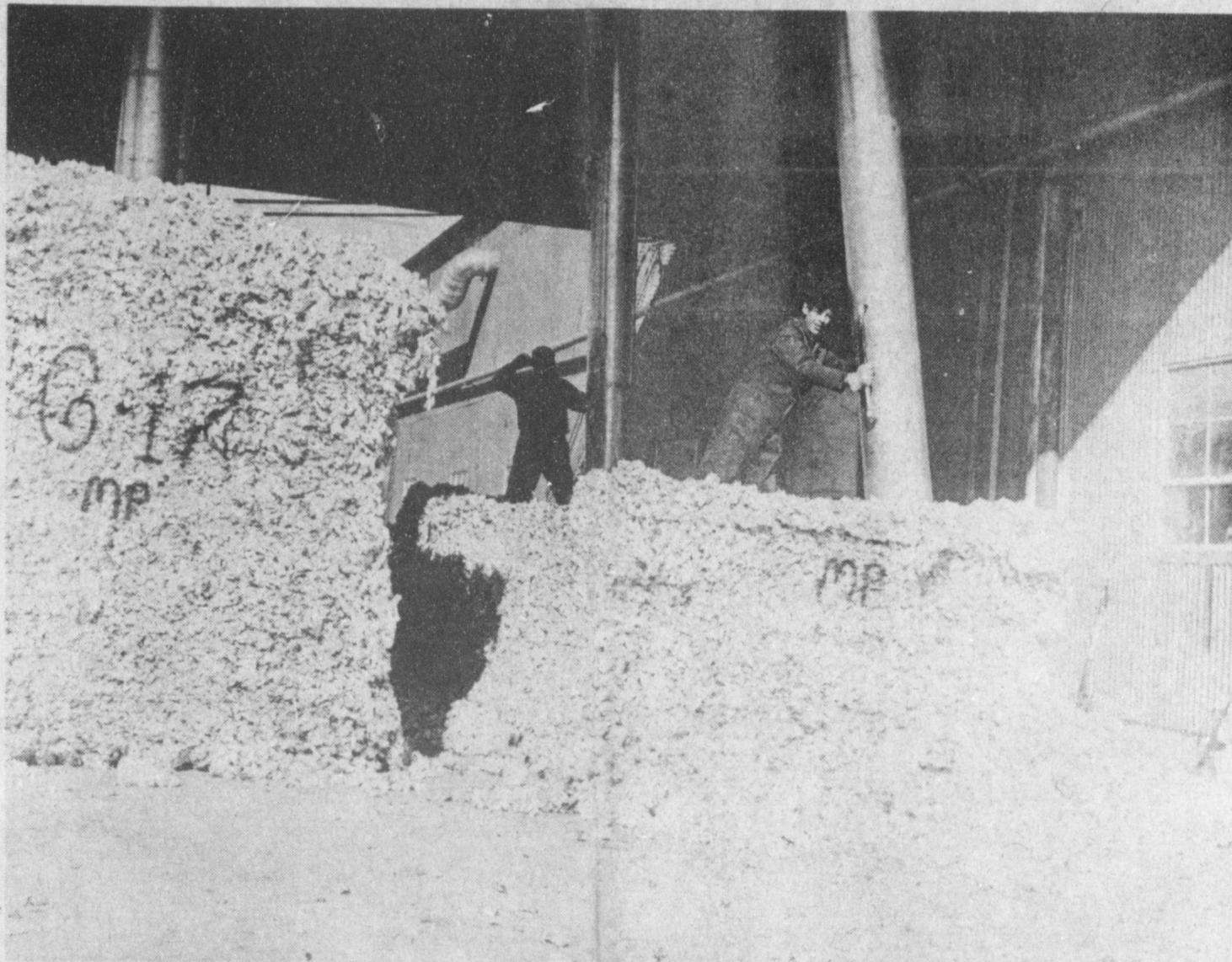
MODULES COMING IN TO THE GIN.... At Muleshoe Co-op Gin on Friday, two workmen were working the suction on modules which are being ginned since snow has kept farmers from harvesting. Ginner Elmer Watson said the gin will handle a module approximately every 27 minutes. From nine to nine and a half bales of cotton are in each module. However, he said they are having to remove the modules at night when the fields and dirt roads are frozen due to the snow and ice.
