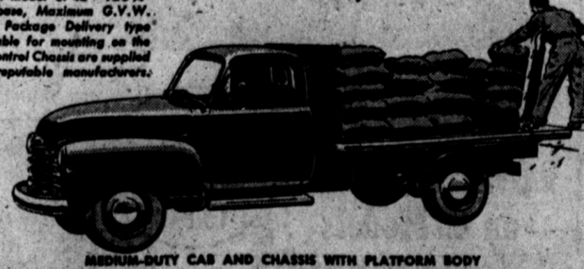
MEDIUM-DUTY CAB AND CHASSIS WITH PLATFORM BODY Model 3808—137-inch wheelbase, Maximum G.V.W. 8,800 lb. Other models available up to 161-inch wheelbase and 16,000 lb. G.V.W.
