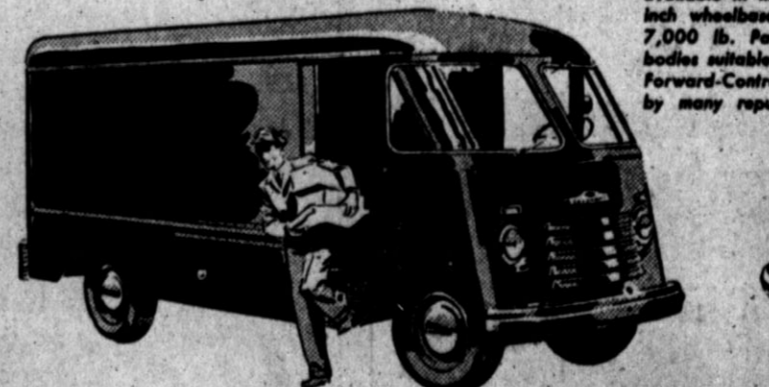
LIGHT-DUTY DE LUXE PANEL* Model 3105—116-inch wheelbase, Maximum G.V.W. 4,600 lb. Also available in Medium-Duty model 3805—137-inch wheelbase, Maximum G.V.W. 6,700 lb.
