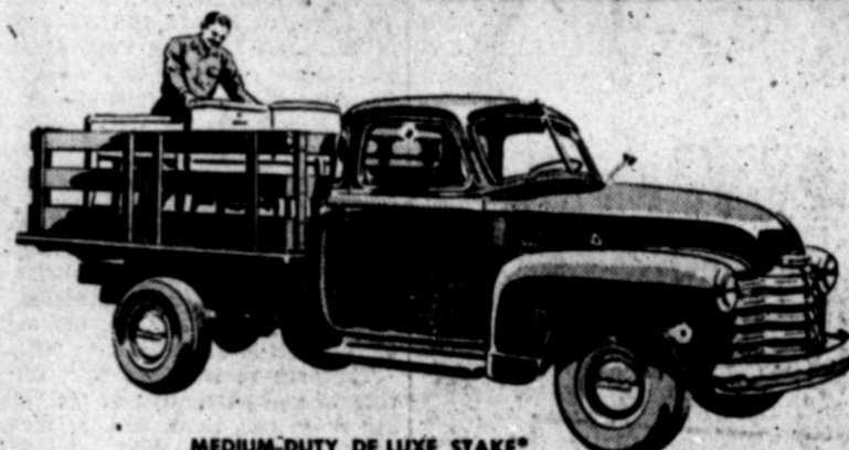
MEDIUM-DUTY DE LUXE STAKE* Model 3609—125 1/4-inch wheelbase, Maximum G.V.W. 5,800 lb. Other models available up to 161-inch wheelbase and 16,000 lb. G.V.W.
