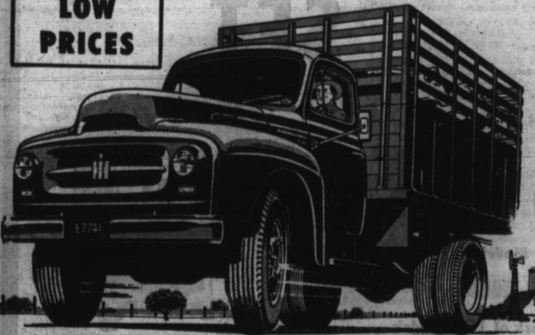
International Model B-160 with combination farm body. B-160 Series, GVW ratings, 14,000 to 17,000 lbs.
