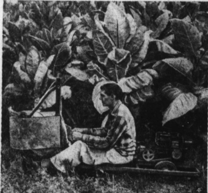
WITHOUT BREAKING his back or the upper leaves from his tobacco, W. C. Hundley rides his low-slung invention through a field, gathering the lower leaves of the plants.
