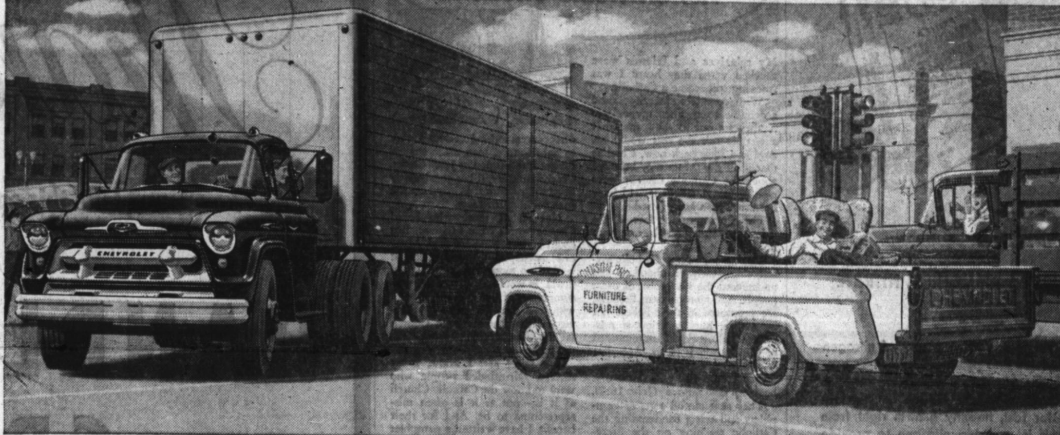
That's one of Chevy's new 8000 Series tandems at left, model 8403. That pickup, model 3604, has an extra-long box (98"), is rated up to 6900 lbs. G.V.W.
