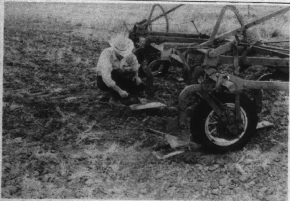
AL LEE, SCS technician examines the 30" sweeps on Charles Hoover's drag type stubble mulch plow. Stubble mulching has become an accepted method of water conservation in Deaf Smith County.
