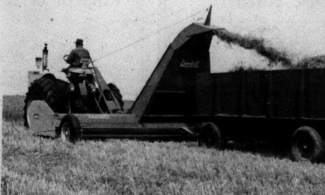
Close the door and the Lundell 804 chopper shredder with the heavy duty cup type cut and throw knife will deliver 6' of material to a trailing wagon.
