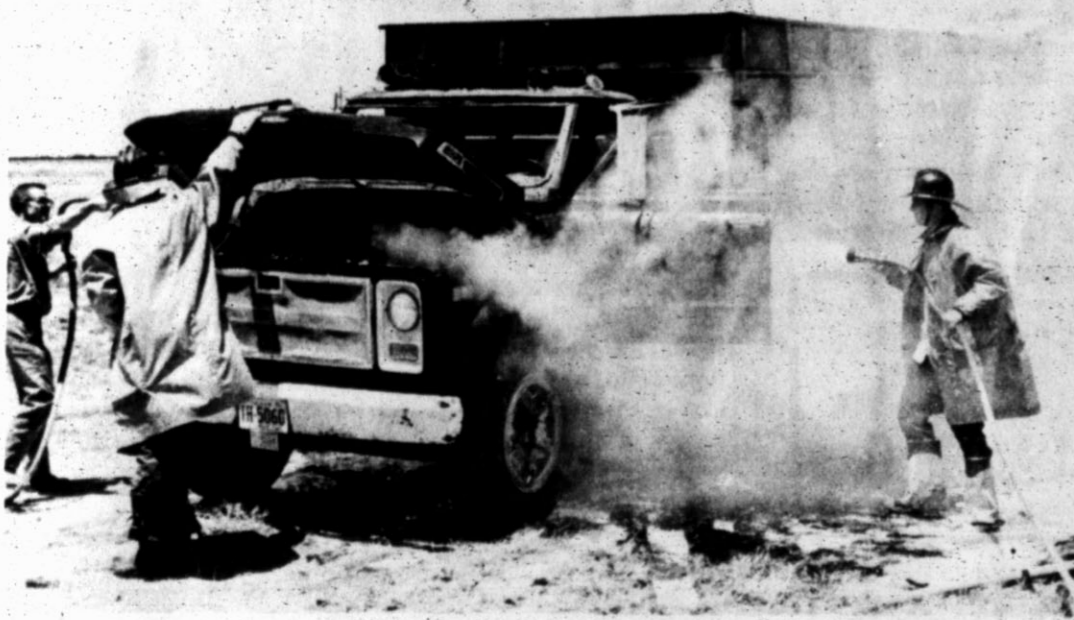
TRUCK DESTROYED — This 1969 Chevrolet truck, belonging to Lawrence Ward Trucking, was destroyed Tuesday afternoon near Summerfield when the electrical wiring under the dash board ignited. The fire spread to the gas tank behind the seat and exploded. Members of the Hereford Volunteer Fire Department arrived at the scene shortly after the alarm was sounded, but the vehicle already was engulfed in flames. Damage was estimated at $8,000.
